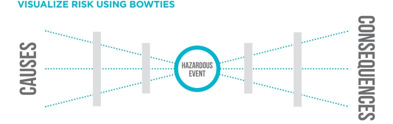
Each Bowtie converts pages of HAZOP data into a single, powerful, easy to understand, graphical visualization, which helps operators understand the full scope of each potential risk, and see the impact of each safeguard.
